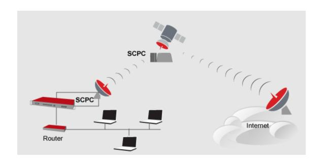
SCPC-based design provides a point-to-point technology, making it the VSAT equivalent to conventional leased lines.
