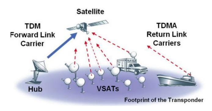
With TDMA networks, numerous remote sites communicate with one central hub – a design that is similar to packet-switched networks In a TDMA network, all VSATs share satellite resource on a time-slot basis.
