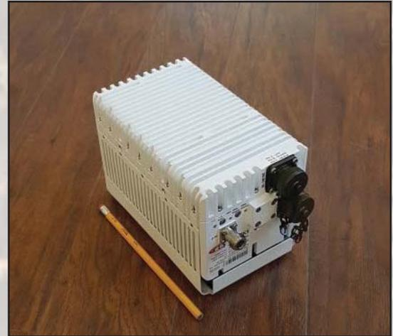
This smallest and lightest 100W L-To Ku-Band Block Up Converter is based on GaN technology. Incomparable low power consumption, double L.O., field-exchangeable connector, auto-sensing and controllable internal 10 MHz reference make this unit universal for any Ku-Band application. M&C (FSK) capability enables troubleshooting, monitoring and controlling the BUC.
