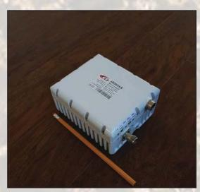
This smallest and lightest 8W L-To Low Ku-Band Block Up Converter is based on GaN technology. Double L.O. and field-exchangeable connector make unit universal for any Low Ku-Band application. Incomparable low power consumption allowes the BUC to be powered by iDirect and similar modems. Internal 10MHz reference option enables using the BUC with the modems without 10MHz reference.
